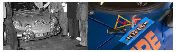
Alpine quickly saw the car's potential in rallying, and segmented the cars into two variants, one for Group 4 and Group 3 rally classes. This example was built for the latter and remains a far closer specification to a regular road car, having factory added roll bars, a circuit breaker, as well as bucket seats and harnesses, a heated windscreen, and perhaps most important of all, a shorter gearbox.
