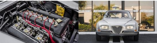
The fully rebuilt engine features high compression pistons, performance cam shafts, and stainless steel tubular headers, so we can only imagine just how good this Italian stallion must sound, especially with its all-important, rare and original Weber intake manifold sporting three Weber 40 DCOE carbs.
