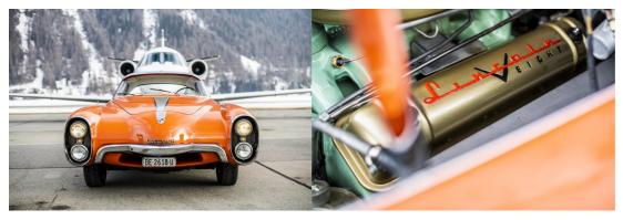
Gian Paolo was thus handed a Lincoln chassis – Lincoln being Ford's luxury marque – and set to work creating large-scale sketches that he and the carrozzeria's skilled craftsman brought to life using a combination of steel tubing and sheet metal. The hugely exaggerated hood was flanked by suitably long wheel arches (or 'fenders' in U.S. speak) that each held twin stacked headlamps and culminated in shrouds from which those fake exhaust tips ostentatiously protruded.
