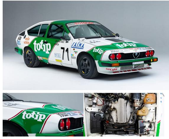
Among the many period modifications done to this Alfa, you'll find a reinforced chassis, a special transaxle close-ratio dog-leg gearbox, alloy wishbones and 'knuckle risers' on the uprights and reinforced torsion bars. These cars also boasted a limited slip differential and centre-lock wheel hubs, along with a modified lightened dashboard.
