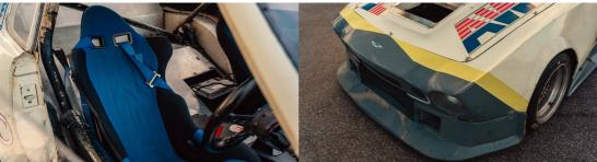
With the mechanical aspects of the car significantly improved, work began on the exterior, where the nose-line was also lowered closer to the tarmac and a different front splitter and spoiler were added for extra downforce. What Jack had created was nothing short of a nightmare for the opposition, and in 1986, Jack and Cousins won the ASCAR trophy in the modified class. Oh, and did we mention they were still running stock brakes?
