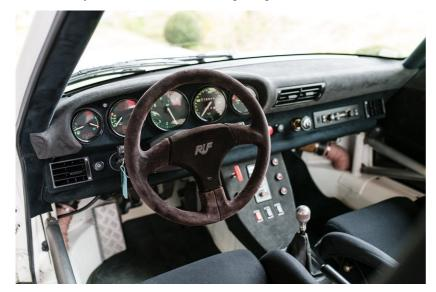
To further show he meant business, Takeyama specified that the car's heater control unit should be shifted to the left in order to allow quick and easy access to the turbo boost control - which sits, enticingly, just a finger's reach from the quick-release RUF steering wheel (which, importantly, is also not far from the ignition isolator switch and plumbed-in fire system...)
