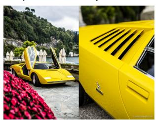
The team at Lamborghini's restoration department decided to recreate the prototype just like it had looked during the show – and to deliberately recreate some of the initial flaws along the way. "The air intakes weren't functional, the degree in which the air enters the engine bay had been calculated wrong – it simply was a mistake", explains
