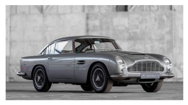
The DB4 Vantage arrived more than a decade later in 1961. In addition to a more potent straight-six engine, which incorporated three SU carburettors and revised cylinder heads, the flagship DB4 boasted faired-in headlights and bright aluminium trim.
