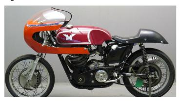
The 500cc Matchless G50 was developed in 1958 by Associated Motorcycles (AMC) at the former Matchless works in London from the highly successful 350cc AJS 7R. Approximately 180 factory G50s were made up to 1963. A race-winning package in the late Fifties, the G50 was lighter than its main competitor the Manx Norton, and as result was often more competitive on tighter, short circuits.
