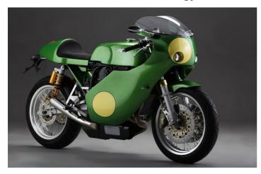
It may take design cues from the past, but beneath that pretty exterior, the Paton S1 Strada incorporates modern technology. The water-cooled, 650cc Kawasaki Ninja engine is used in conjunction with a six-speed gearbox, propelling the bike up to a max speed of 215km/h. And it could readily be used as a 'daily rider'. Available in four trim levels, the S1 Strada will be priced from 16,000 euros, with a limited 'Factory Signature' variant costing 23,000 euros. Now pull your tongue back in...
