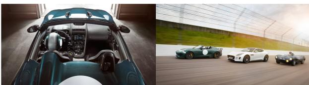
It's the differences from the standard [F-type Roadster](#) that are most impressive: a headline 575HP, up 80HP from the V8 S; a substantial 80kg weight reduction, achieved with the extensive use of carbonfibre elements; 177% more wind-tunnel-honed downforce; and an even more sonorous soundtrack from the active exhausts (as if improvements were needed in that area).
