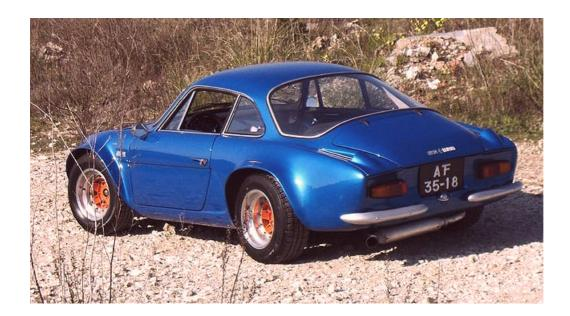
The combination of grunty, rear-mounted, four-cylinder engine and short, exploitable wheelbase made the might Alpine A110 the ideal machine to tackle the twisty mountain roads above Athens. No wonder it conquered the Acropolis three times: in 1970 and 1973, under Jean-Luc Thérier's control, and in 1971 with Ove Andersson at the wheel.
