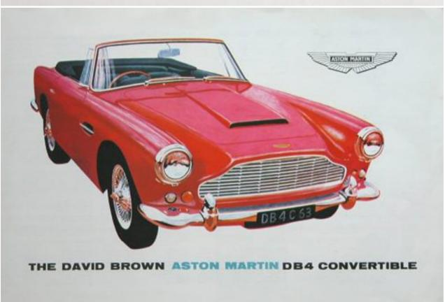
The DB4 was an instant hit. As fast and stylish as any Ferrari or Maserati, it soon became a favourite of the wealthy sporting motorist – and this was despite early setbacks of multiple engine failures, eventually solved by nearly doubling the oil capacity and adding an oil cooler.
