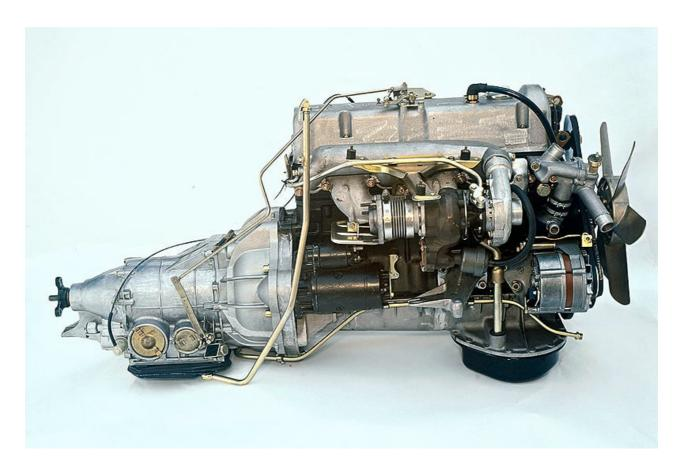
From May 1978, the W116 model range welcomed the 300 SD engine, a forerunner of today's familiar luxury diesel. The 3.0-litre five-cylinder diesel-engined version came complete with a turbocharger – Europe's first turbodiesel – and was initially tested in the C111 experimental vehicle (top picture).
