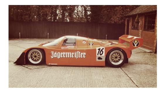
Thanks to its flamboyant Jägermeister livery, this 962C already has plenty of visual impact. The 'art' is in keeping the car in running order (engine rebuilds are required every 3,000km), so that it can do what it does best: crafting pretty arcs on the racetrack.
