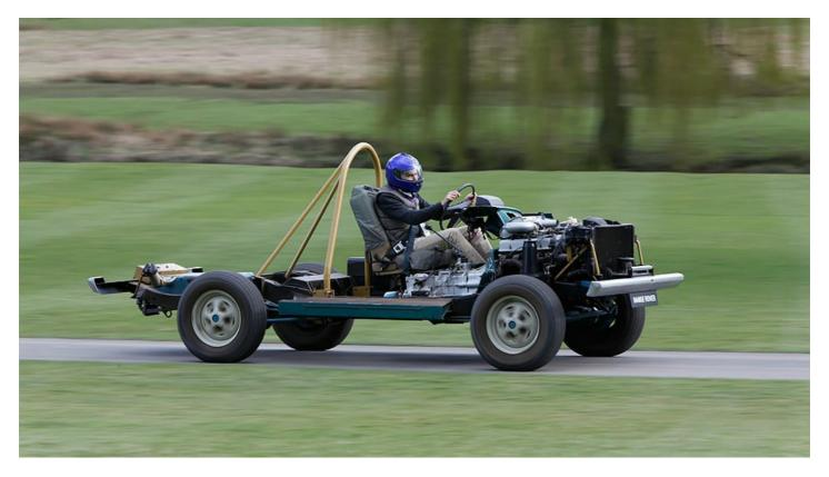
Range Rovers have that touch of luxury, eh? Not this one. We tried off-roading in the demonstration chassis from the first production Range Rover and the thrill of seeing the coil springs working and the propshaft turning half-convinced us that not only is it possible to do without air-con and audio system, but you don't really need a body at all. It just spoils the fun.
