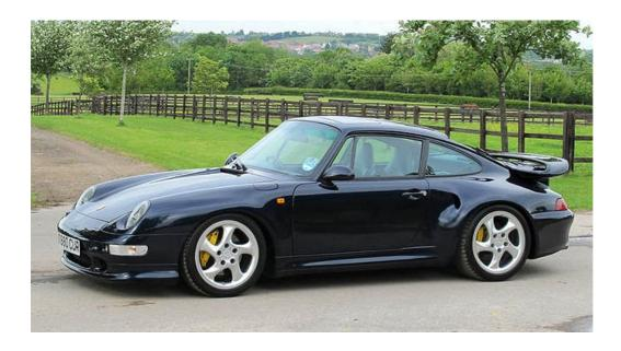
The third-generation Turbo was launched in 1995, and encompassed technology originating from the 959 supercar – namely the use of two turbochargers and a permanent all-wheel-drive system. As with some of the later 964 Turbos, an 'S' derivative was subsequently offered; just 183 were produced, all benefitting from a hike in power (to 444bhp in non-American markets) and differentiated by their yellow brake calipers, 959-style rear arch scoop, four-pipe exhaust system and larger spoiler.
