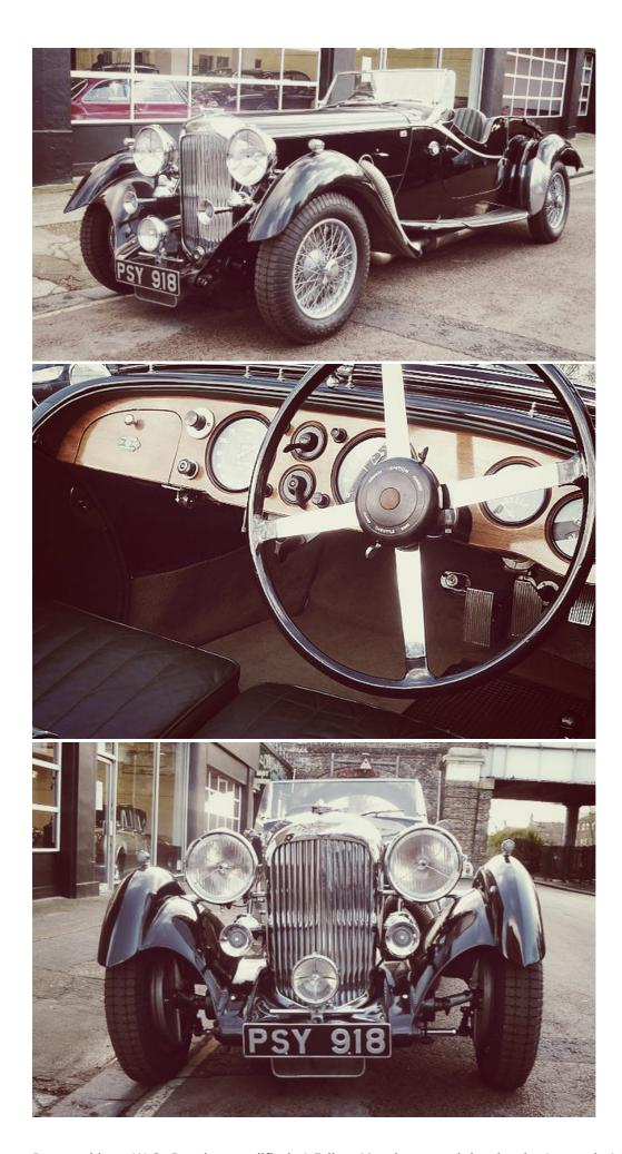
Powered by a W.O. Bentley-modified, 4.5-litre Meadows straight-six, the Lagonda LG45 was the spiritual successor to the 'Cricklewood' Bentleys. The company had won at Le Mans in 1935, and to stress its sporting
