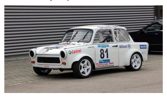
Getting on for 3 million Trabant 601s were made during its 27-year production run, but this one certainly stands head and shoulders above the rest – in performance terms at least. It's equipped with a 1300cc Suzuki Hayabusa superbike engine in place of the usual 595cc two-cylinder, while the wider track should help to control its newfound performance a little better.
