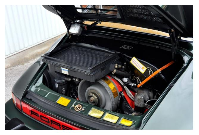
Yet the car's inner values remain the same: a 3.3-litre air-cooled boxer engine with turbocharging and intercooling, paired with a four-speed manual gearbox driving the rear wheels. At the time, the 911 Turbo was purely a RWD model – it was nearly two decades before the model gained 4WD.
