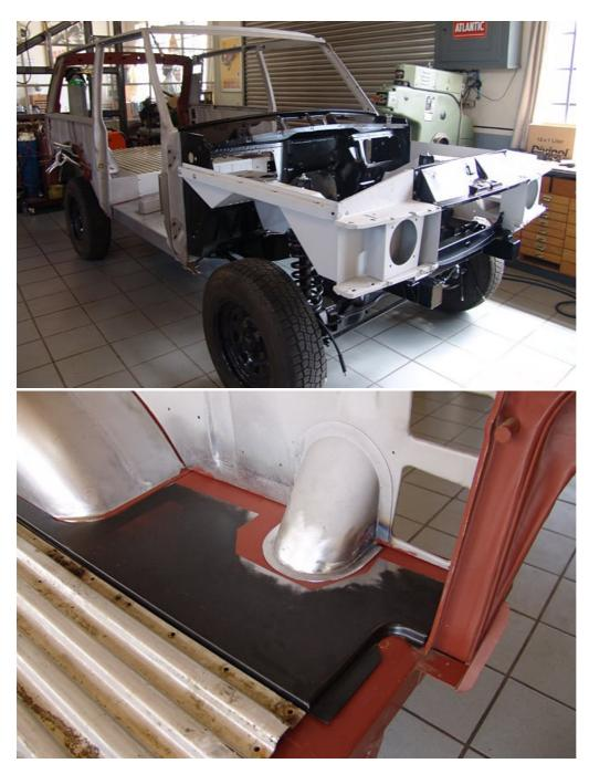
While the turbo engine is transported to a specialist for renewal, LandyPoint takes care of the axles, suspension, brakes and transmission. The chassis is also sandblasted and renovated, then remarried to the body and sealed.
