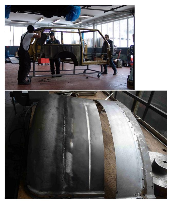
The workshop team at LandyPoint has over 20 years' experience in Range Rover restorations, and can take a Classic right down to its last bolt – then all the way back up again. Unlike the Defender, the Range Rover has a skeletal steel frame with aluminium body panels flanking the exterior. As a result, rust can only be identified if the body panels are removed. Corrosion often lurks behind the coachwork of even the most outwardly-flawless examples.
