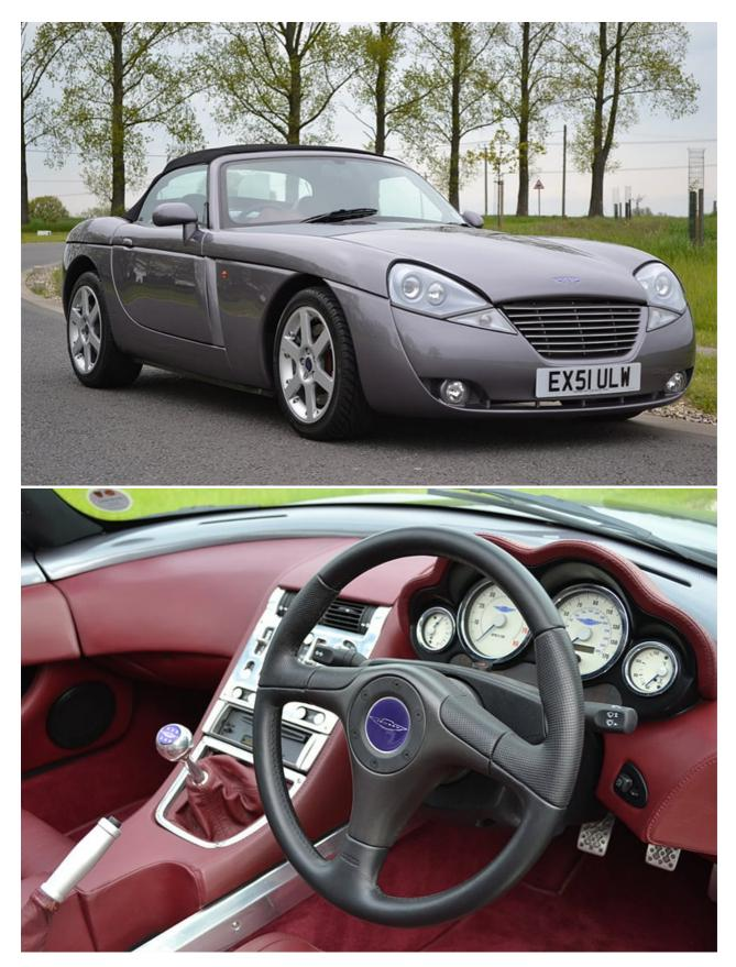
The SV-8 programme certainly started with a bang. Benefiting from £10m in investment funding, the distinctly styled convertible (by Howard Guy and Gary Doy) was built in Merseyside and launched at the 1998 British Motor Show. It was powered by a 4,601cc, 32-valve, four-cam, V8 Ford Mustang engine, producing 325bhp and promising to speed the car to 60mph in under five seconds and on to a top speed of 160mph.
