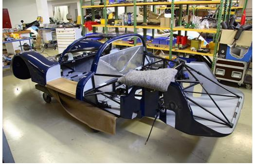
After the race, 906-017 was totally stripped down and the spidery tubular chassis tested for cracks. Suitably reinforced, with yet more lessons learned, it was sent to Sicily as a training car for the forthcoming Targa Florio. This proved to be very tough, as the factory drivers pounded round and round the tough Sicilian road course... which was not closed to the public.
