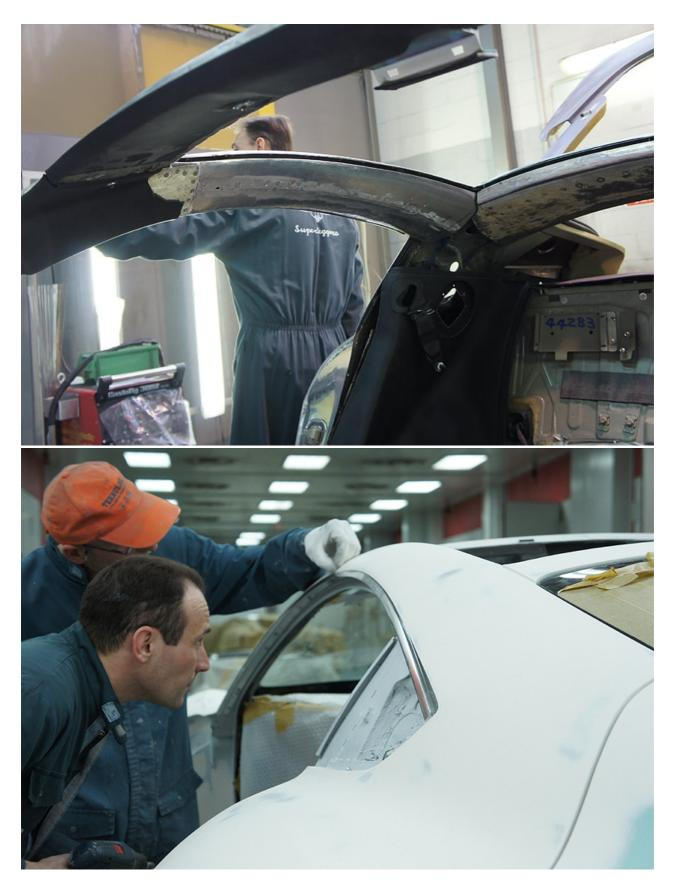
The car is now ready to be painted. First, all panelwork is meticulously filled, smoothed and given a coat of primer.
