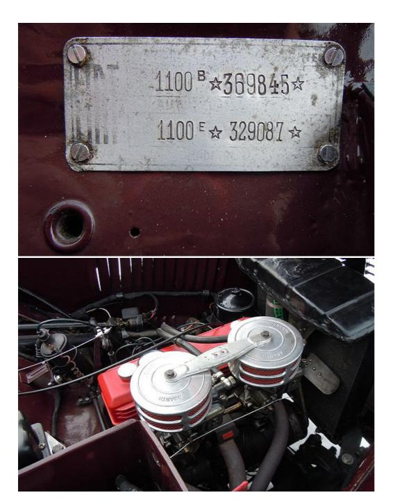
Under the bonnet sits an Abarth-tuned four-cylinder engine. With a special cylinderhead and twin carburettors, the small car has the typical high-revving performance of the period.
