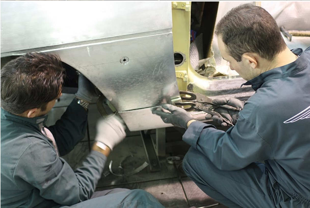
As we said before, this is Italian metalworking technique passed down from generation to generation. No 'English wheel' here - it's all beaten, sometimes by hand, but mainly with the aid of a power hammer, to faithfully follow the lines of the mock-up.
