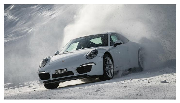
It's a simple calculation: the weight of the car (say 1,500kg) is multiplied by the theoretical grip of the road (perfect traction will equal '1.0') and you then get the available braking force, in this case 1,500kg. When it rains, the multiplier reduces to 0.7. In snow it's 0.2 and in wet snow 0.1. Factor in a downhill slope and the braking forces are negligible. Welcome to the new Porsche 911 Carrera 4S, *Bienvenue au Col de la Croix*.
