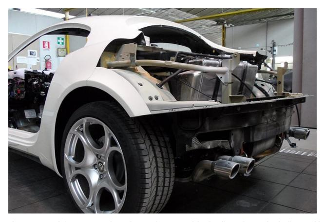
The sequence of photos you see here shows a donor 8C arriving in Milan. It is completely disassembled – apart from the chassis, drivetrain and all mechanical parts. All components to be used later are carefully labelled and stored, and the wiring loom partially removed.
