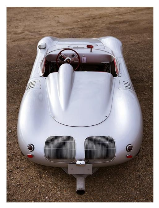
The RSK made its debut at the 1957 Nürburgring 1000Km. It differed from the preceding 550A by having large-choke Weber carburettors (over 140bhp was now available at 7500rpm), a new space-frame chassis, lower, more streamlined bodywork with an Appendix C (to meet the governing body's latest rules) windscreen, bigger brake drums and revised suspension front and rear.
