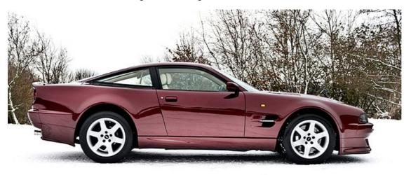
Normally available as a six-speed manual (with automatic conversions offered post-purchase by Works Service), it was a very fast car. Speeds approaching 200mph are talked about, and the sight of a V550 on full throttle is akin to watching a Phantom or Lightning embarking on a Cold War emergency scramble. Officially, a 186mph top speed is promised, with 60mph coming up in 4.6 seconds from standstill.
