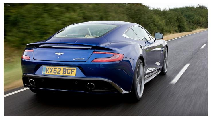
At the tail we find a spoiler flying above the main boot surface but moulded seamlessly into it, while around the body's lower edges the splitter, diffuser and lower sills parade their carbonfibre in glossy nakedness. Bumpers remain in deformable plastic.
