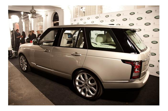
The list of engineering achievements is stellar. And lengthy. How about a body-in-white that weighs less than the equivalent of a new BMW 3 Series? The all-aluminium body and sub-frames have helped the car shed up to 420kg against the previous car – that's the equivalent of five passengers.
