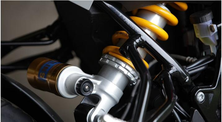
Like the engine, the frame is also from the F800, but it's been tweaked for added strength and greater agility. The Husky 900 and 900R share many of the same major components and, apart from a few carbonfibre trinkets, the R also boasts top-spec Brembo front brake calipers and adjustable suspension – Sachs front and Ohlins rear.
