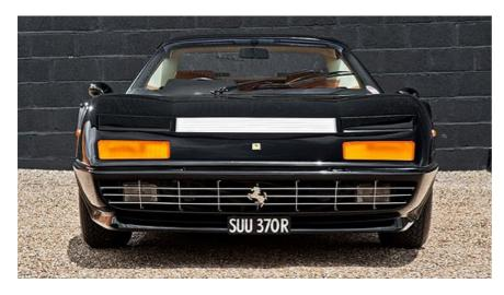
Named '512' after the earlier racing Ferraris, and referring to its (near enough) 5-litre engine and 12 cylinders, with 'BB' standing for 'Berlinetta Boxer' (technically wrong; it has a 180° V12), it arrived in 1976 as an improved version of the 365 GT4. The main alterations from its predecessor included an increased engine capacity (up to 4942cc), revised rear suspension, wider wheels, and some subtle visual changes.
