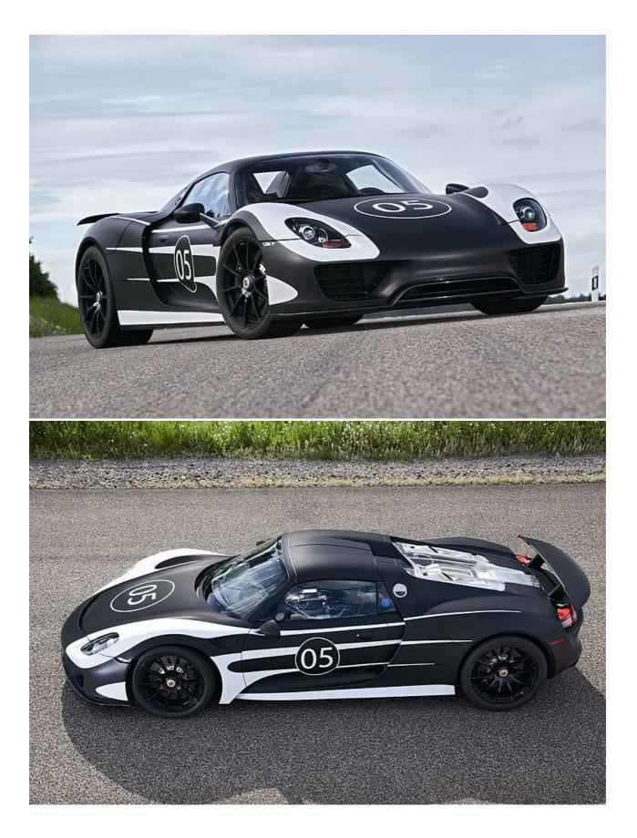
At the heart of the modern miracle is a 4.6-litre V8, mounted amidships and joined by a hybrid module on the rear axle (which also has adaptive steering) and an electric motor on the front axle. The technological showcase continues with a full carbonfibre reinforced plastic (CFRP) monocoque, fully adaptive aerodynamics, and an upward-venting 'top pipes' exhaust system.
