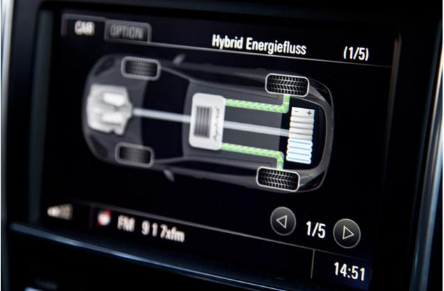
We could no doubt help the fuel economy along by learning to drive in a more 'eco' manner. For example, the battery under the boot floor is recharged during braking, and this regenerative braking can be tracked on the central display – Bonus Points and Miles collectors will love this feature, and the more you practice, the better you get.
