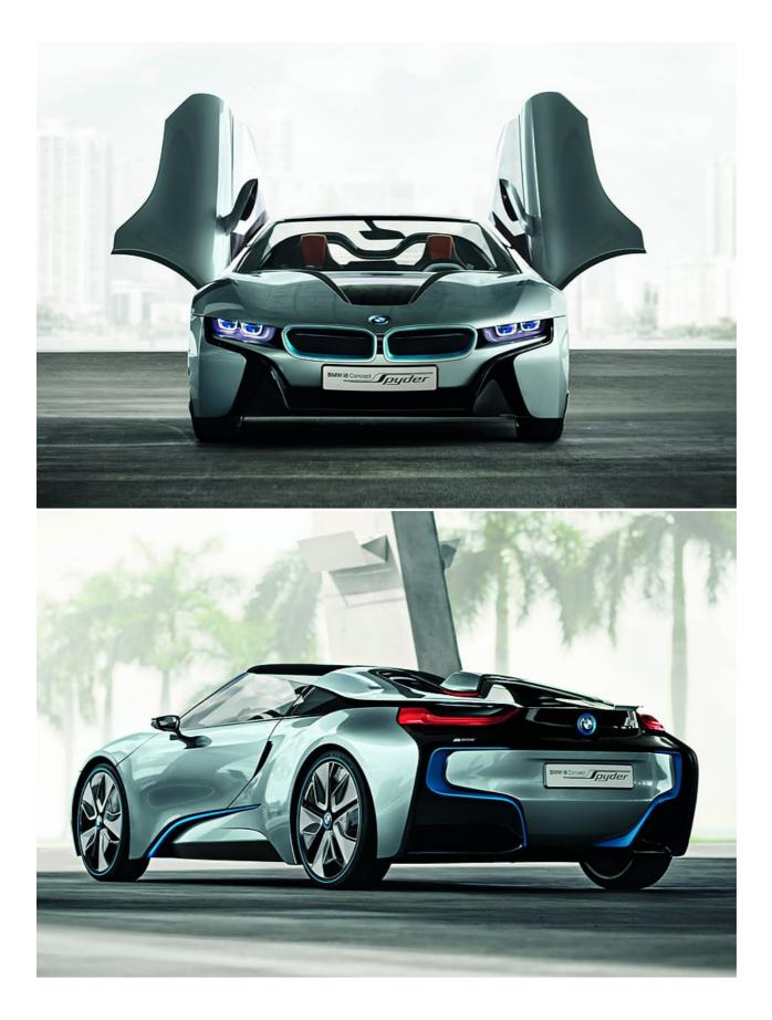
The 4.4m-long and 1.9m-wide i8 Spyder stands just 1.2m high, making it as low as a Ferrari 458 Italia. Despite the lightweight concept with extensive use of CFRP (carbonfibre reinforced plastic), the BMW comes in at a hefty 1.63 tonnes. Adding to the weight is the high-capacity battery, fitted low to keep the centre of gravity as close to the ground as possible.
