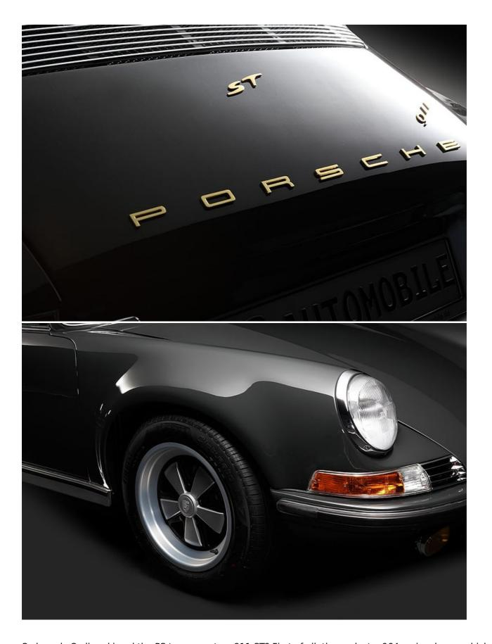
So how do Sadlowski and the PS team create a 911 ST? First of all, they select a 964-series donor vehicle, the penultimate air-cooled 911. This is then totally dismantled and the body fitted with the ST's front bumper and characteristic flared front and rear wheel-arches (an 'RS-style' front spoiler is an option). New indicators, fog lamps and chromed headlamp surrounds are installed. The bonnet is glassfibre – as per the original ST.
