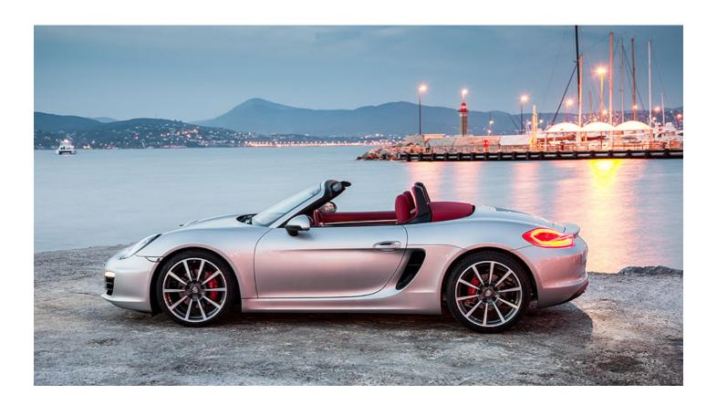
What is undeniably an advantage is a 40 per cent increase in the structure's torsional stiffness, thanks mainly to high-strength steels in vital places, including a boron mix for the sills. The skin panels and the floor are aluminium, and the whole car weighs between 25 and 35kg less than its corresponding predecessor.
