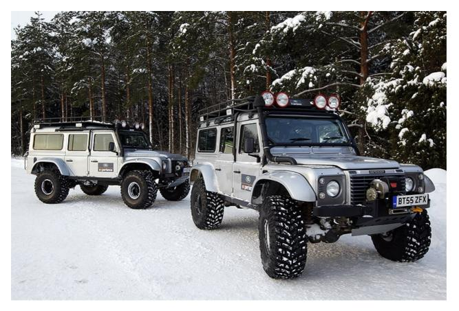
The team at Land Rover Special Vehicles modified the chassis quite extensively to accommodate the wheels and diff lock compressors, although the turning circle remains significantly greater than standard. Other extras include long-travel dampers, anti-roll bars, a detachable chassis cross member, snorkel, Warn winch, interior roll cage, auxiliary cabin heater, GPS and satellite telephone.
