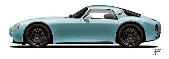
In the standard Coupé, the diesel produces around 200bhp and 300lb ft of torque, which means the 1121kg car is good for a 0-62mph sprint of around 5.6 seconds. The slightly heavier (1159kg) petrol-engined standard car has a similar twist figure, but cranks up the power to 300bhp – thus reducing the sprint to 62mph from standstill to just 4.3 seconds.
