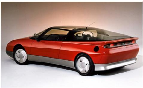
The EV-1's modernity continued above its waistline: the roof was made entirely of bronze-tinted, heat-resistant glass embedded with solar cells – the latter of which powered an interior cooling fan, a concept revisited by the latest Audi A8. Only the narrow A-pillar and less-narrow, chassis-reinforcing targa bar thwarted a panoramic view of the outside world, though their blackened state gave the car a futuristic appearance. A host
