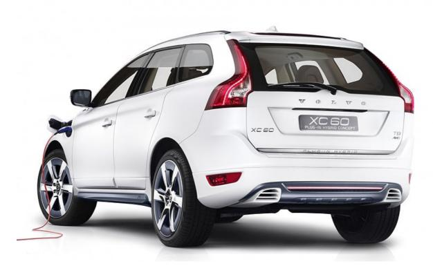
Three different driving modes are present in the concept XC60 (and in the production V70): Pure, Hybrid and Power. Pure uses electric power only, while voltage is used to increase economy in Hybrid mode and performance in the Power setting. To aid thriftiness, the drivetrain only operates in four-wheel-drive mode in low grip situations.
