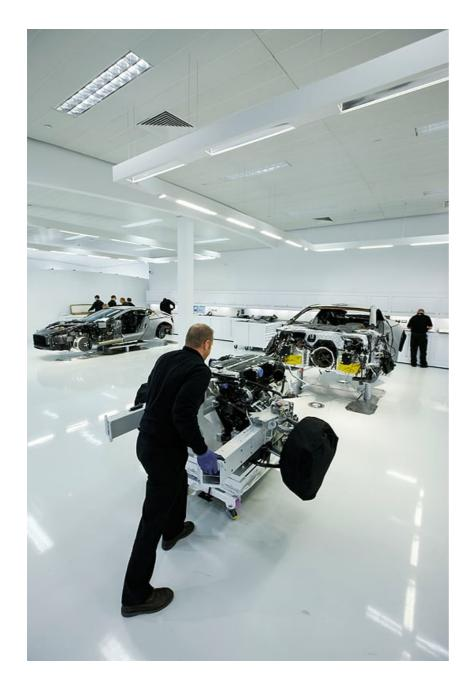
With the immensely tough chassis and lightweight composite parts stripped down, then painted and reassembled in the main factory, it's time for the car to be built up by hand in the One-77 building, where drivetrain, brakes, all plumbing, wiring and trim is carefully installed.
