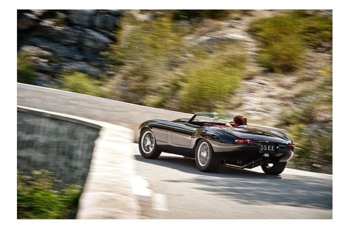
Built on an original E-type chassis, the Speedster has a subtly redefined body made entirely from aluminium; its alloy engine, a specially developed version of Jaguar's legendary six-cylinder XK unit, has been bored to 4.7 litres and produces around 310 horsepower which is delivered to the specially made rear wheels through a bespoke, five-speed, aluminium gearbox and aluminium diff.
