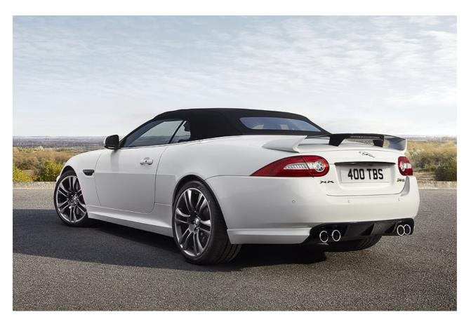
Wider wheels, forged for lightness, complete the mechanical modifications, while the body gets a new nose with slots ahead of the bonnet, a carbonfibre splitter and side ducts which channel air along flared-out sills. Carbonfibre forms the new rear wing and lower valance too, all designed for extra stability and reduced lift at high speeds.
