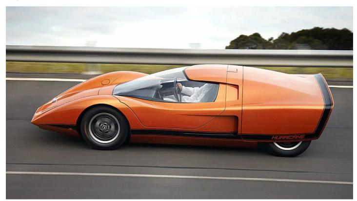
Entry to the 39-inch-tall concept came via an electro-mechanical canopy, which pivoted forwards to reveal the two seats, that in turn rose to 'greet' the soon-to-be occupants. Once cocooned inside, the drama changed from visual to aural as the 262bhp, 4.2-litre V8 burbled into life, before whisking away whoever was lucky enough to pilot the one-off Hurricane. Occupants were kept safe by the inertia-reel seatbelts, and comfortable by the climate control system.
