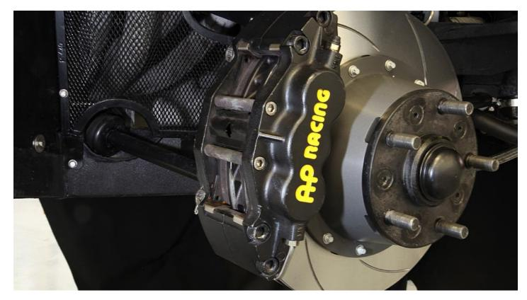
The first option ('Kit 1') is a four-piston caliper coupled with a 304mm, straight-cut grooved disc. This can be fitted to all V8s produced from the early 70s to the end of production in 1989.
