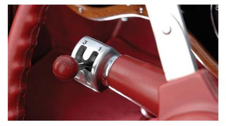
So, to set off, the procedure is as follows: depress clutch, select 'forward', select first on the steering-column 'gate', release handbrake to driver's right, release clutch – with a whiff of throttle, it's got tremendous torque – and off you go. So far so good. By the way, you have four reverse (as well as forward) gears available to you, but third is usually selected when backing-up.
