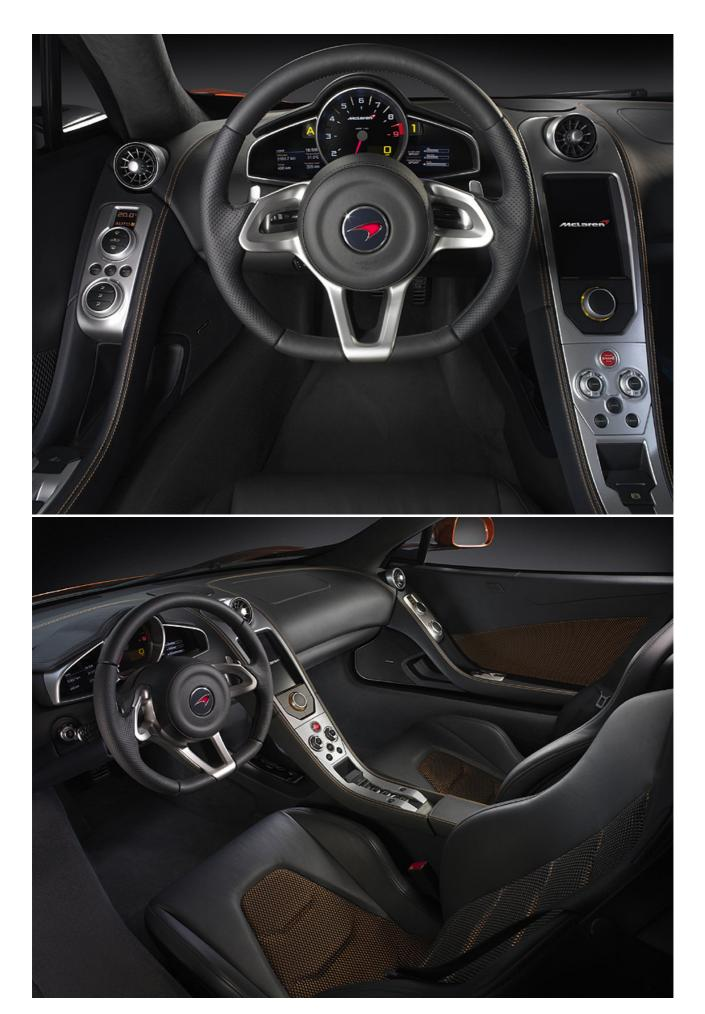
The functional but beautifully finished interior contains no parts from other cars; every component is special to the MP4-12C. Like the original **McLaren F1**, many controls have been moved to the most ergonomic positions, such as the armrests of the doors.
