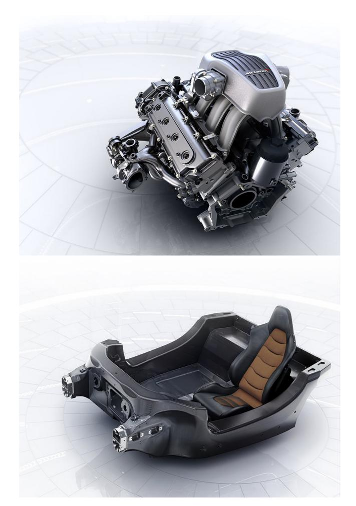
Powering the car is a **twin-turbocharged, 3.8-litre 90° V8 engine** (redlined at 8500rpm) developed entirely by McLaren, one that will produce 600bhp and 600Nm torque. 80 per cent of the latter is available below 2000rpm, so it's extremely flexible as well as more powerful than the recently announced **Ferrari 458 Italia**.
