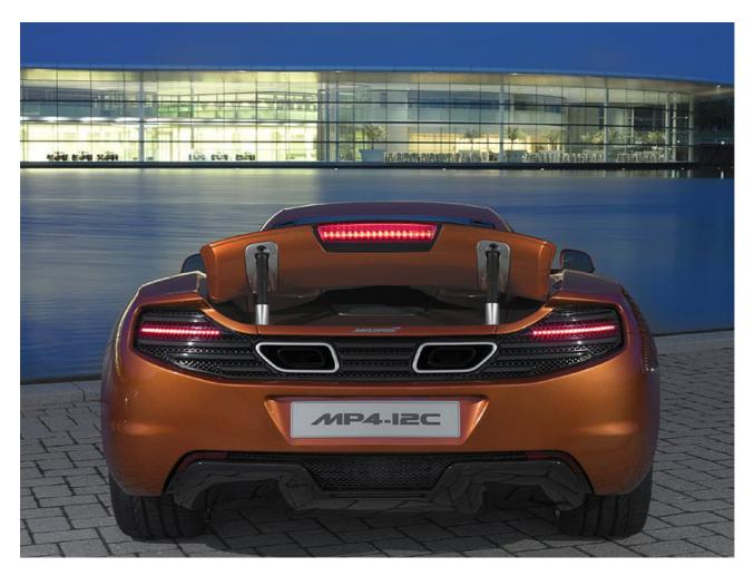
The biggest hint from the McLaren F1 is at the rear, with a sloping 'glasshouse' engine cover and slightly pushed-forward rear lights. Like the older car, it also has dihedral-opening doors and the aforementioned airbrake.
